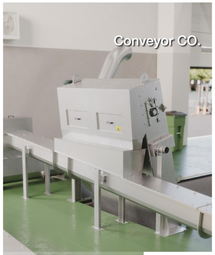
Conveyor CO conveys screenings, sludge, sand and waste either by spiral screw or by flushing.
